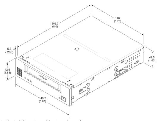
**Figure 7-1** Physical dimensions of the internal tape drive
